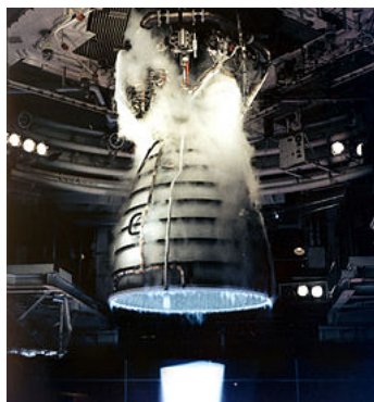
The Space Shuttle Main Engine burnt hydrogen with oxygen, producing a nearly invisible flame at full thrust.
